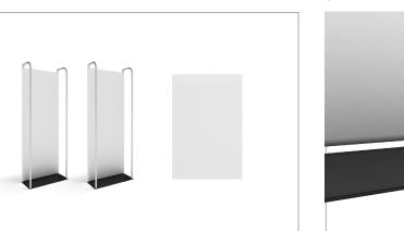
**Step 2:** Assemble post (75) into the outside hole of the two connecting base plates shown in illustration. Screw by hand, turning post to tighten into place.
