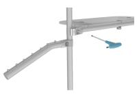
(OPTIONAL) To add shelves or accessories to frame, position and level part on frame before tightening clamps down with hex tool.
