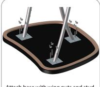
Attach base with wing nuts and stud. Insert threaded rods by hand.
