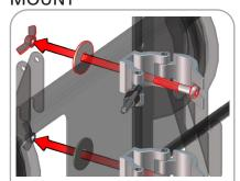
Attach ACC60 clamps to monitor mount with a bolt and washer, tighten with wingnut.
