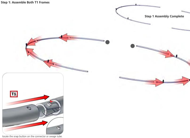
locate the snap button on the connector or swage tube. Locate the hole on the corresponding tube. Press the snap button with your thumb and slide the tube and connector together so that the snap button snaps fully into the lock hole. To disassemble, press the snap button and pull apart.
