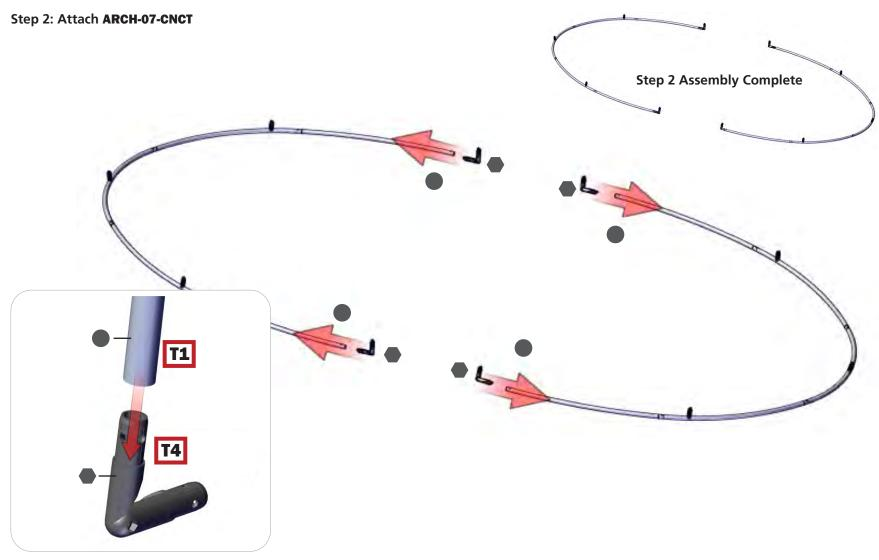
Snap in ARCH-07-CNCT connectors at all ends of the arches. use the provided hex key tool to loosen the corner screw for adjusting the angle of the connector to fit your frame. Next, take the plastic connector and make sure the snap buttons are in proper position for the frame tube holes. Simply press the snap button with your thumb and carefully slide the tube onto the connector. The snap button should pop through. Some twisting may be necessary to assure the snap button has
