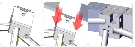
The scissor frames will have middle hubs installed on all four sides front and left and right sides of back. Attach the middle caps of the channel bars onto the middle hubs. The middle caps of the channel bar will snap into place.
