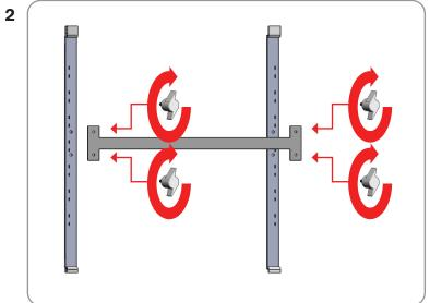
Assemble the mounting hardware by attaching the bar to the brackets - align the holes and use the included screws.
