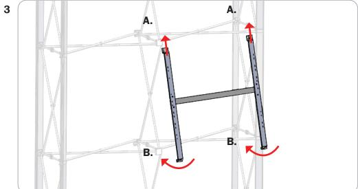
A. Attach the bracket assembly to the Embrace frame by first tilting it up and attaching the top of the scissor brackets to the upper embrace arms. Make sure brackets are the correct orientation before attaching. Follow the strickers on the brackets.
