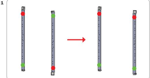
Locate the stickers on the accessory brackets and turn them so they are rotated to the correct direction.
