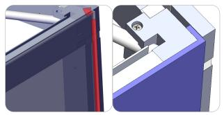
As an optional feature, the front printed graphic may have end cap graphics with silicone edge. Pull the end cap silicone edge to the top of the back corner hub. Start to press in the SEG into the hub and work your way down the side channel. Do the same for the opposite end cap.
