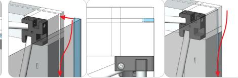
To apply the silicone edge graphic, start by pressing the SEG into the top left corner hub of the frame. Continue to press the SEG into the extrusion bar fabric channel. Keep pressing the SEG into the bar fabric channel until you make down to the bottom right corner hub of the frame. This also works for the opaque liner or the second printed graphic option on the back side of the frame.
