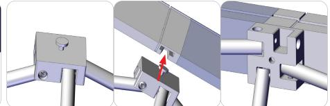
The scissor frames will have middle hubs with a metal prong installed on all four sides front and left and right sides of back. Attach the middle caps of the channel bars onto the middle hubs. The middle caps of the channel bar will snap into place.
