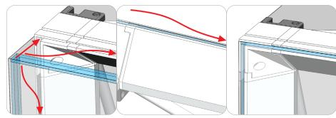
To apply the silicone edge graphic, start by pressing the SEG into the top left corner hub of the frame. Continue to press the SEG into the extrusion bar fabric channel. Keep pressing the SEG into the bar fabric channel until you make down to the bottom right corner hub of the frame. This also works for the opaque liner or the second printed graphic option on the back side of the frame.
