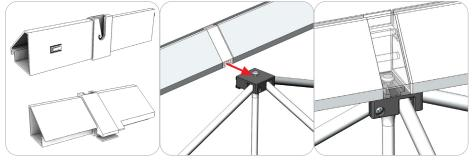
The back-lit scissor frames will have middle hubs with a metal prong installed on all four sides front and back. Attach the middle caps of the back-lit channel bars onto the middle hubs. The middle caps of the channel bar will snap into place.
