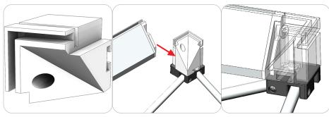
The back-lit frames will have this corner hub installed on all four corners, front and back of the frame. This corner hub takes the end caps of the back-lit channel bars. The end caps of the channel bar will snap into place.
