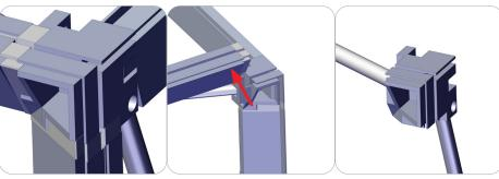
To remove the channel bars, start by pulling the end caps off the corner hubs.
