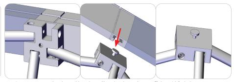
Continue to remove the channel bars by pulling the channel caps off the middle hubs.
