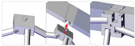
The scissor frames will have middle hubs with a metal prong installed on all four sides front and left and right sides of back. Attach the middle caps of the channel bars onto the middle hubs. The middle caps of the channel bar will snap into place.
