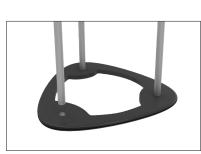
**Step 6:** Turn counter upside-down. Pull graphic taut and angel and tuck gasket into channel in edge of base. Insert graphic gasket all the way around.
