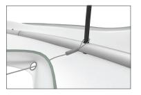
**Step 8:** Zip graphic closed around top of frame. Pull all cables out until inside loop is flush with eyelets. Attach all cables together at a single point for hanging.
