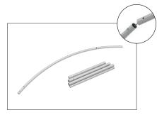
**Step 6:** Align top frame to bottom frame and push support poles into the frame. With some force connect the support poles in the middle to complete.
