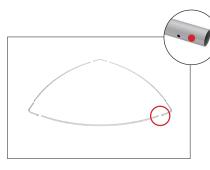
**Step 7:** Unzip print and place one frame inside. Position holes on frame to align with eyelets in graphic. Thread cable through eyelet. Repeat for all eyelets.
