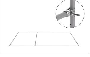
**Step 5:** Attach foot onto corners of frame to connect together.
