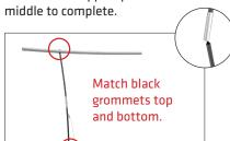
**Step 7:** Unzip print and place one frame inside. Position holes on frame to align with eyelets in graphic. Thread cable through eyelet. Repeat for all eyelets.
