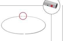
**Step 7:** Unzip print and place one frame inside. Position holes on frame to align with eyelets in graphic. Thread cable through eyelet. Repeat for all eyelets.
