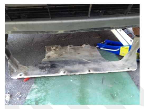
Now remove the screws along the bottom of the bumper cover, 3 larger ones across the center and 3 smaller ones at each side.
