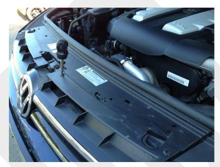
Then gently ease the grill forwards so you can look down and see the plastic clips that run along the bottom of the grille so you can see how they attach; I recommend spraying some silicone down onto the clips to assit in prising them out.
