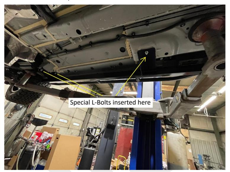
Front seen with the large nutsert installed. Also, L-bolt installed on the right side.
