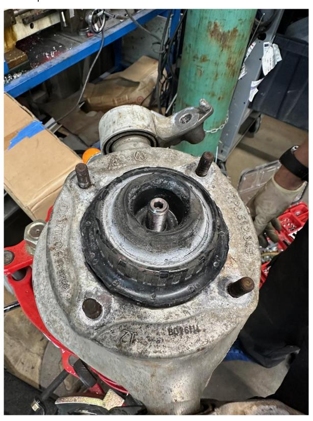
Install the OEM rubber mount on then install the provided nut and tighten to 45ft lbs.
