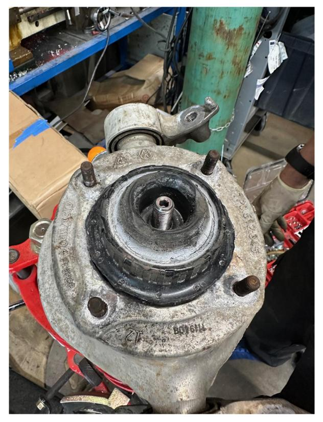
Install the OEM rubber mount on then install the provided nut and tighten to 45ft lbs.
