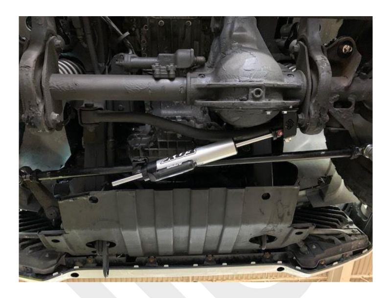
5. Install the large bolt on the differential side next. You can torque this bolt completely at this time.
