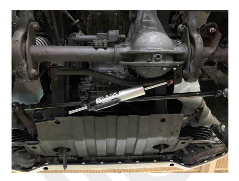
5. Install the large bolt on the differential side next. You can torque this bolt completely at this time.
