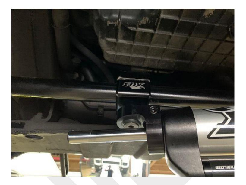
4. If you measure from the end of the locking nut at the pitman arm. You will be approx. 12.5 inches from end to end. this will cause no binding issues turning lock to lock from left to right.
