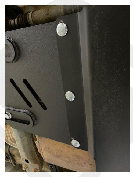
Carriage bolts face upwards to keep from damaging the hardware. Lock nuts are installed on top.
