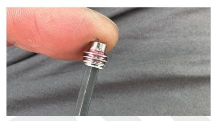
The sleeve must be low as possible with access to the set screw. If it's not low enough the knob will not have engagement on the shifter.
