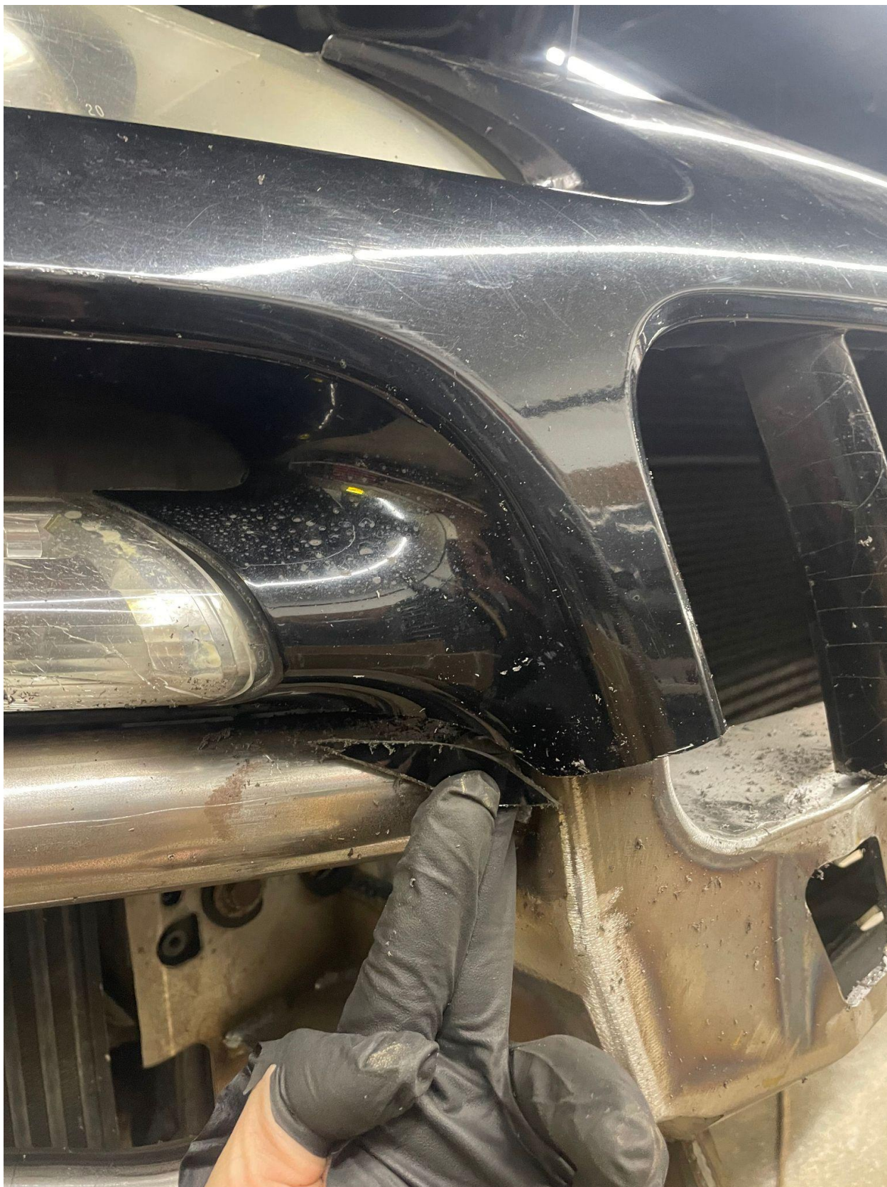
Trim edge of bumper cover near turn signal housings to clear tubular side bar.
