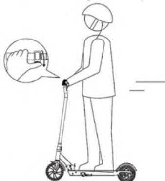
6.Press the left handle button to brake. When the speed is too fast, the left foot can step on the rear wheel fender for auxiliary braking. Be careful not to press the brake button too hard, otherwise it will cause a sudden brake.
