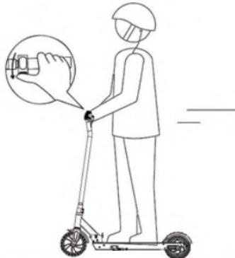
4.Gently press the accelerator button of the right handlebar to drive slowly, and turn the handlebar to control the riding direction (similar to bicycle).
