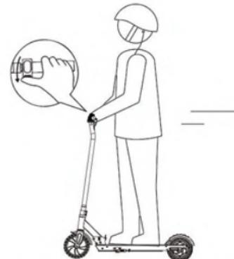
5.Lightly press the accelerator button on the right hand, the car can accelerate, remember not to be too fast.
