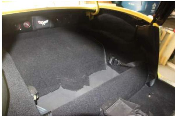
Lay the single sheet of HushMat Silencer Megabond over the wheel well with the white release paper intact. Measure and cut with scissors or utility knife. Peel back one straight edge of the white release paper and adhere the Silencer Megabond directly on top of the HushMat Ultra on the Wheel Well. Repeat this step for both wheel wells. Silver or black foil performs exactly the same.
