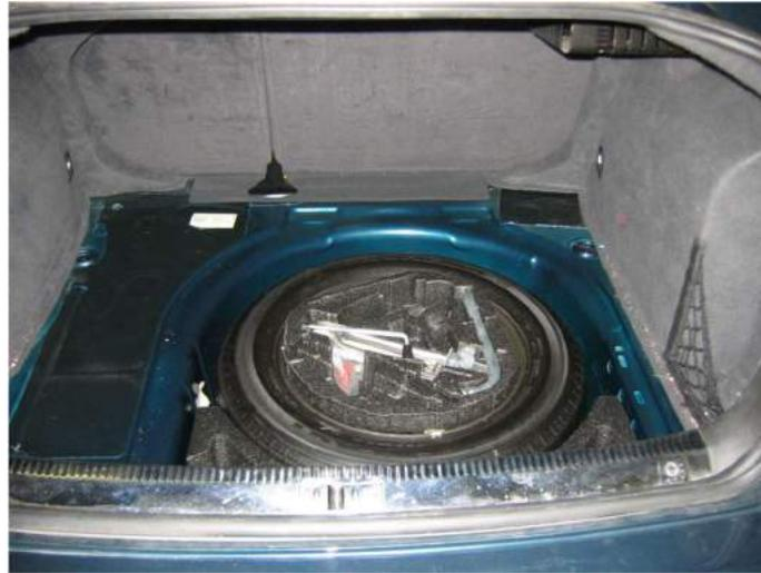
Note: images below illustrate both our black foil and silver foil material, they exhibit the exact same performance characteristics – the only difference is the black ink will apply to the foil so it does not reflect light. Remove all plastic and fabric trunk trim and spare tire (on many vehicles you may be required to remove the rear seats to reach these areas). Vacuum loose dirt, sand or dust from the sheet metal surfaces.
