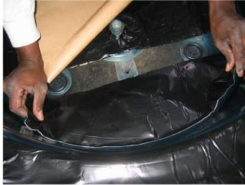
Repeat the above step until you have covered the floor and rear wall of the trunk. A good tip is to save any small cut outs or pieces of the HushMat Ultra for patching smaller areas of the trunk.
