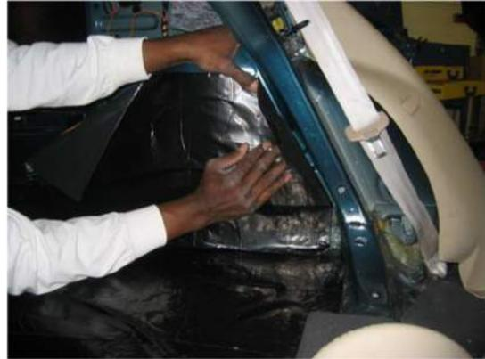
Peel back the brown release paper and press the sheet onto the wheel well starting at one edge and work your way across the well. Apply consistent hand pressure across the sheet working the material into any ribs or groves in the sheet metal.
