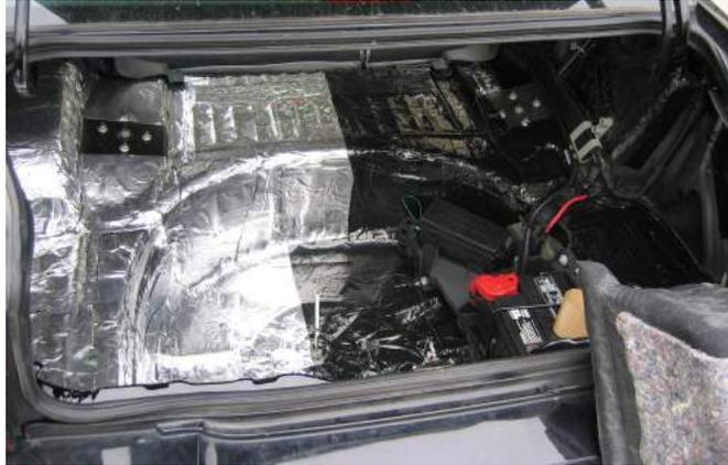
Treatment of the rear quarter panels is required due to the thin gauge sheet metal and the small amount of interface with the vehicle frame. These expansive panels are loosely supported and resonate. Cut the large sheet of HushMat Ultra in half and press it onto the inside of the outer quarter panel skin through the frame.
