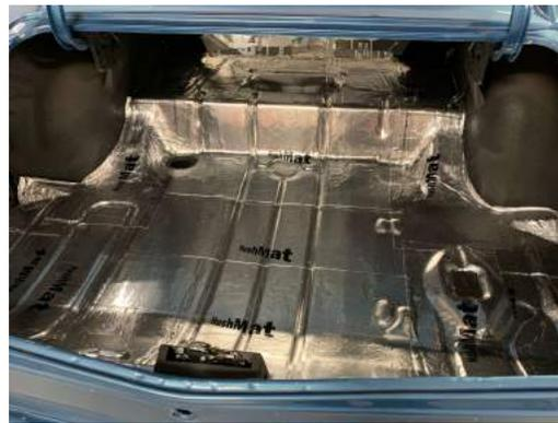
*The above provides an installation guide for your vehicle. The Trunk kit covers the area from the point under the rear set, covering the wheel wells, trunk floor, rear quarter panels and spare tire well. The images and schematic are not intended to reflect the exact dimensions of your Make, Model and Year vehicle.*
