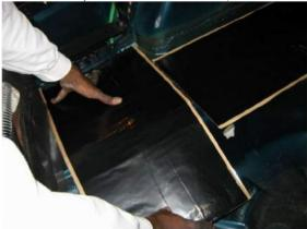
Prior to removing the brown release paper, place the sheet of HushMat Ultra damping material across a straight edge of the trunk beginning against the quarter panel wheel well of the vehicle to determine adequate fit or "nesting". Cut the sheet to fit the space if necessary, with scissors or utility knife prior to peeling back the release paper.
