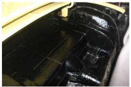
We recommend 100% coverage is recommended for optimum acoustic & thermal performance of the trunk area. The space from the rear well to the driver/passenger is a determining factor. The shorter the distance between the driver/passenger seat to the trunk the greater the noise level and annoyance factor from road, tire and aftermarket exhaust.
