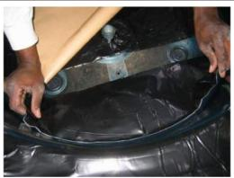
Repeat the above step until you have covered the floor and rear wall of the trunk. A good tip is to save any small cut outs or pieces of the HushMat Ultra for patching smaller areas of the trunk.
