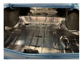
The above provides an installation guide for your vehicle. The Trunk kit covers the area from the point under the rear set, covering the wheel wells, trunk floor, rear quarter panels and spare tire well. The images and schematic are not intended to reflect the exact dimensions of your Make, Model and Year vehicle.
