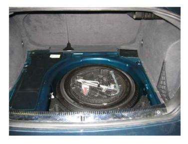
Note: images below illustrate both our black foil and silver foil material, they exhibit the exact same performance characteristics – the only difference is the black ink will apply to the foil so it does not reflect light. Remove all plastic and fabric trunk trim and spare tire (on many vehicles you may be required to remove the rear seats to reach these areas). Vacuum loose dirt, sand or dust from the sheet metal surfaces.
