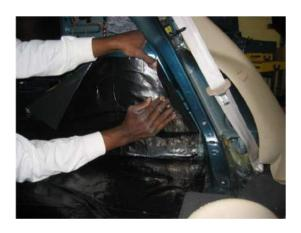
Peel back the brown release paper and press the sheet onto the wheel well starting at one edge and work your way across the well. Apply consistent hand pressure across the sheet working the material into any ribs or groves in the sheet metal.
