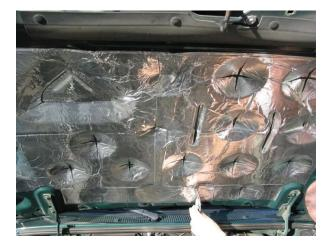
Apply each sheet of HushMat Ultra directly on the metal surface and use light hand pressure to allow material to form into uneven surfaces or channels. If the hood has deep draw areas you can cut cross patterns with a razor knife to allow the material to form into the bottom of the draw. Reinstall the fabric/fiber mat.
