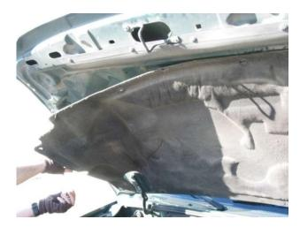
Start by removing the fabric mat from underneath your hood. The fabric mat is typically fastened with push pins and can be reinstalled.
