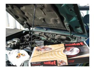
HushMat Hoodliner is formulated to insulate/reflect heat away from your hood. The Hoodliner kit contains 12 Square Feet of approximately 1/8<sup>th</sup> inch thick 0.6 pounds per square feet heat insulating material. This kit is designed to treat a full size or truck hood. HushMat Hoodliner performs up to 550 degrees F (288 C). Hoodliner is paintable.
