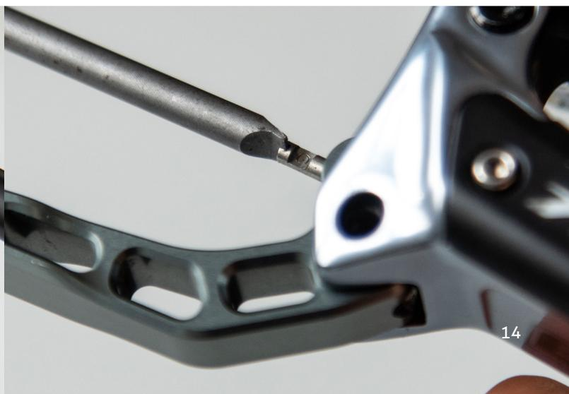
Press the pin back into the transmitter housing and the TRL Brakelever from above. Note the mounting direction of the pin, it must be pressed in with the end with two grooves first.
