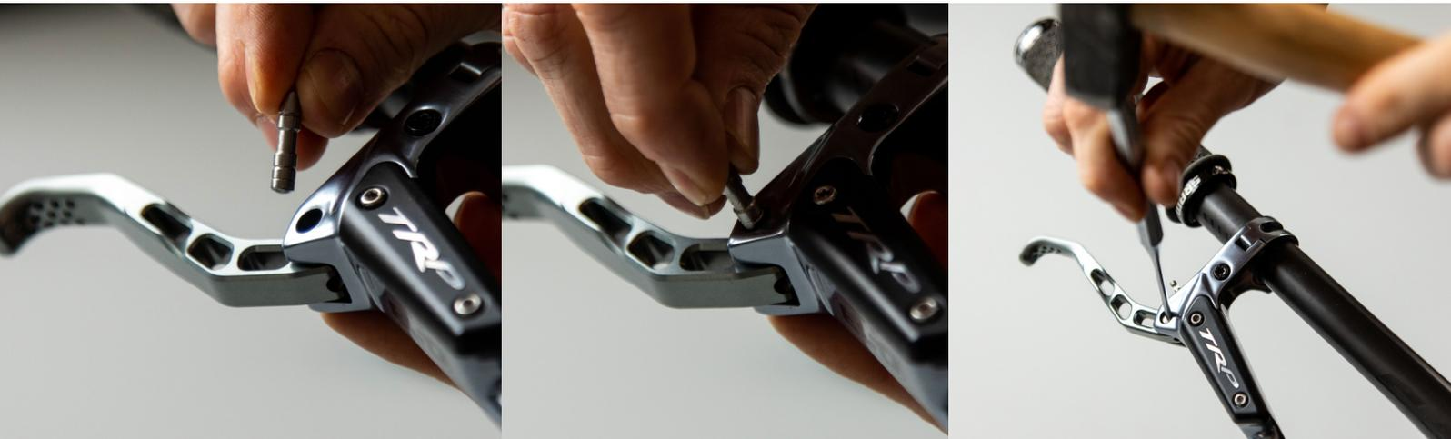
Now put the adjusting knob back onto the thread of the lever reach adjustment and tighten the set screw hand-tight. Align the adjusting knob so that the set screw clamps the flat surface on the lever reach adjustment.
