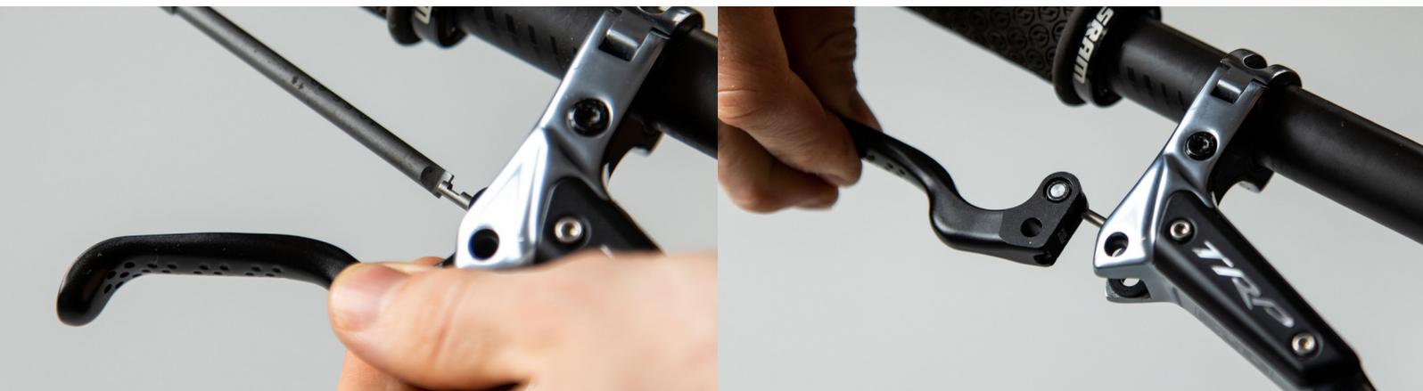
Note: Make sure that the lever bushings do not fall out of the transmitter housing. If the lever bushings no longer hold in the transmitter housing, you can reattach them in the transmitter housing with a little grease.
