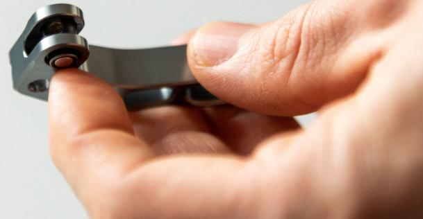
Slide the TRL Brakelever back into the transmitter housing. Thread the detent mech bushing onto the thread of the lever reach adjuster. Screw the thread of the lever reach adjustment back into the detent mech bushing using the screwdriver.
