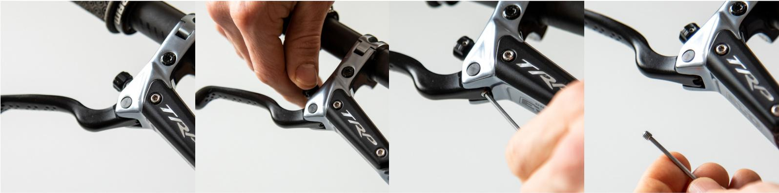
Now loosen the set screw on the adjustment knob of the brake system and pull it off.
