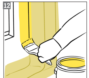
12 Apply additional coats of Liquid as necessary.
