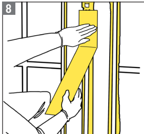
8 Cut Tape and apply to smooth surfaces separated by a seam.
