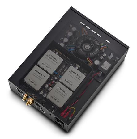
power duties within so that the environment is quieter in terms of electrical noise. Both the Vega S1 and Purer-Power S1 have linear supplies but the one in the external box is bigger and thus has an easier job running the processors inside the Vega S1.
