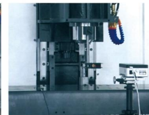
激光镭射检测及校正补偿 Laser detection and correction compensation
