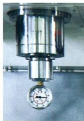
主轴拉刀力检测 Spindle broach force detection
