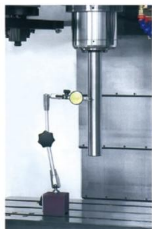
主轴偏摆精度检测 Spindle deflection precision detection
