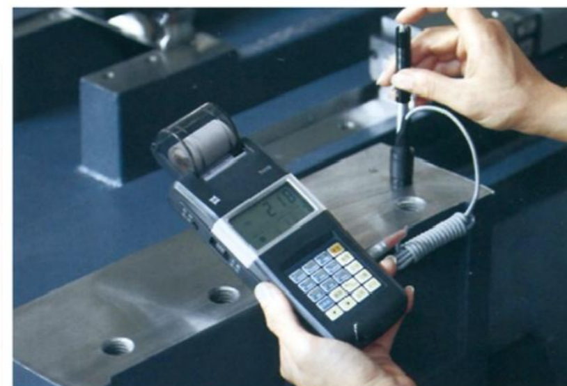
铸件硬度检测 Casting hardness testing
