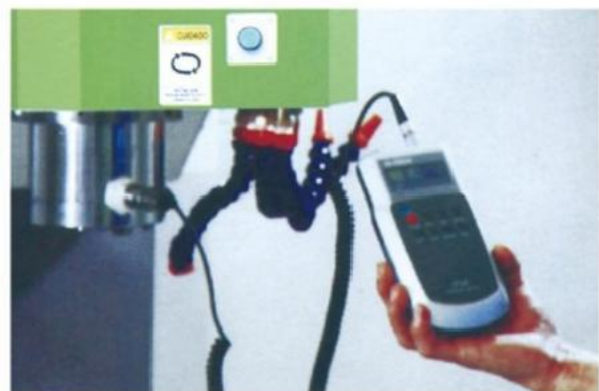
主轴震动检测 Spindle vibration detection
