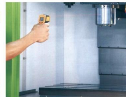
主轴温度及温升检测 Spindle temperature and temperature rise detection
