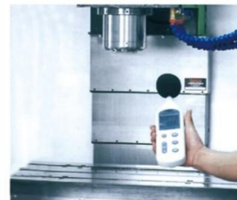
主轴噪音检测 Spindle noise detection
