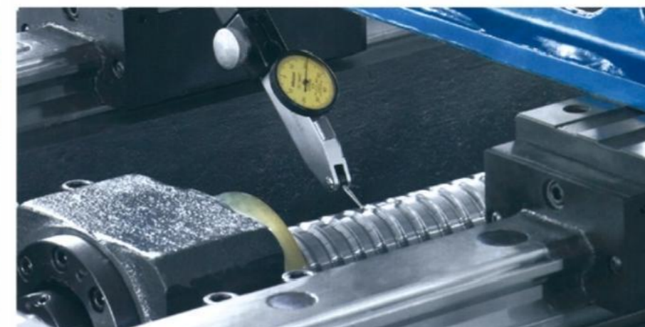
丝杆平行度精度检测 Screw parallelism precision detection
