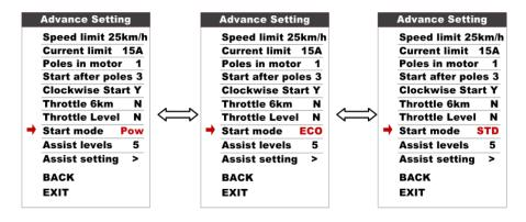
**2.6.23** Assist levels: This parameter can customize assist levels, options are 3/5/9/UBE, UBE represent factory default settings.
