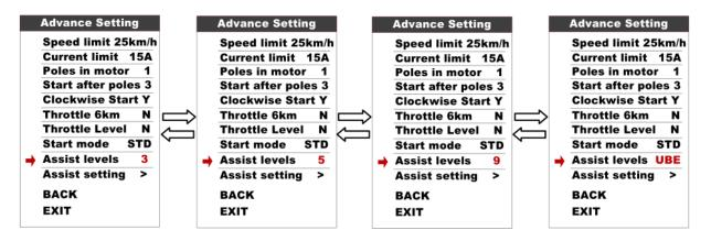
**2.6.24** Assist Setting: This parameter can customize assist ratio.
