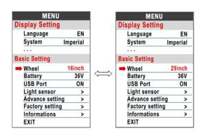
**2.6.11 Battery**: Press UP/DOWN will change battery voltage setting, optional value is 24V/36V/48V/UBE, UBE means user define value.
