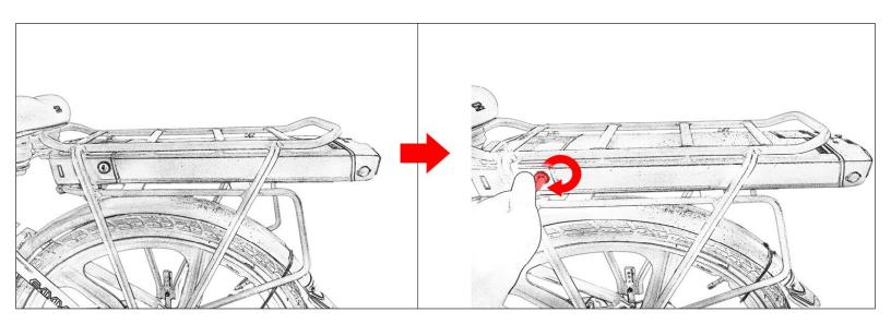
· Hold the tail part of the battery and slide the battery out carefully.
