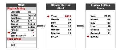
**2.6.9 Start password**: Press POWER button get into the password setting menu. If you turn it on, you must input right password before powering it on. To set the password, press UP/DOWN to change the number and press POWER to switch to the next digit.
