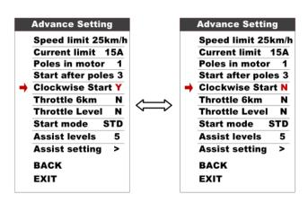
**2.6.20 Throttle 6KM**: this parameter can set the throttle function, N represent max speed, Y represent 6km/h.
