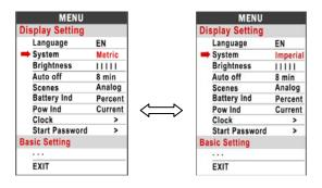
**2.6.3 Brightness**: Press Up / Down button to change the brightness of the backlight, I is the dimmest, IIIII is the brightest.
