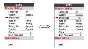
**2.6.4** Auto off: Press UP/DOWN button to change the auto power off time, from 1 to 9, the number represent time (in minutes) to shutdown, default value is 5 minutes.
