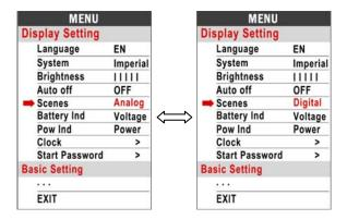
**2.6.6 Battery Ind**: Press UP/DOWN button to change the battery indicator, Voltage / Percentage / OFF.
