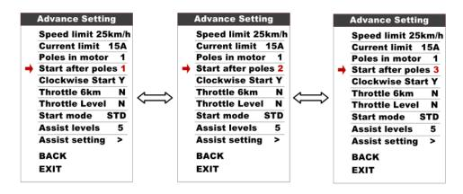
2.6.19 Clockwise start: This parameter represent speed sensor turning direction, default value is Y (forward).
