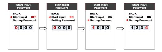
You need to input the correct password within 30 seconds, the display will power off automatically if the password is wrong.
