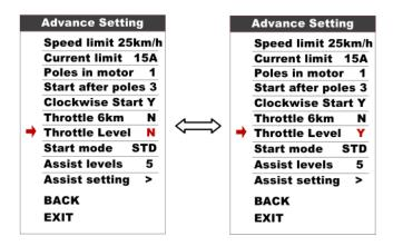
2.6.22 Start mode : Pow/ECO/STD(default) represent Power/ECO/Standard, Power mode means use maximum current when speed up, ECO mode means use minimum current.
