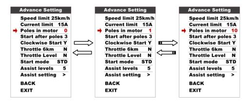
**2.6.18 Start after poles**: How many poles (speed sensor) need to be detected by controller before starting motor. Default value is 3.
