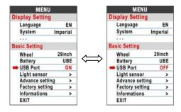
**2.6.13 Light sensor (Optional)**: Press the UP/DOWN button to turn ON/OFF the sensor. Press the POWER button to switch to sensitivity setting. You can change between **HI/MID/LO**.
