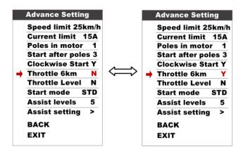
2.6.21 Throttle Level: This parameter is only valid when Throttle 6KM is set as N, Press UP/DOWN will change Y/N, N represent Throttle start max speed, Y represent throttle's speed is related to the assist level.
