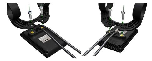
Clamps suit for 3 size of handlebar, 31.8mm, 25.4mm, 22.2mm, there are transfer rings for 25.4mm and 22.2mm, transfer ring must be assembled with the special directions, pay attention to the green arrow below.
