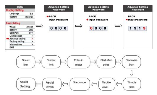
2.6.15 Speed limit: Press UP/DOWN will change the speed limit.
