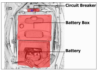
The circuit breaker is located on the front wall of the battery compartment (Internal organization could be different for different ent battery configurations).
