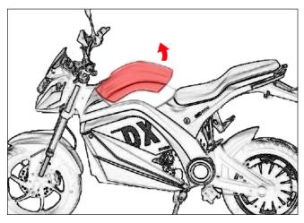
While keeping the storage lock in the unlocked position, gently lift the gastank cover up.
