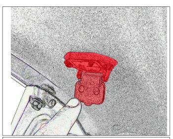
To charge the bike, open the charging port lid and plug in the charger.
