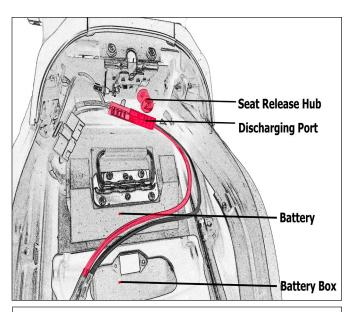
To open the seat, there is a hub (a 'Z' letter on it) behind the battery. Simply pull the hub, and the seat will be unlocked.
