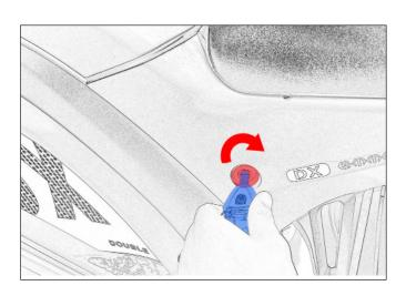
Turn the key in the direction as indicated to unlock the storage tank.
