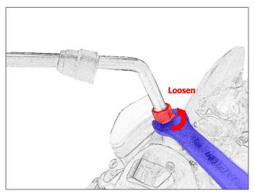
Use the wrench and follow the direction indicated to loosen the nut slightly.
