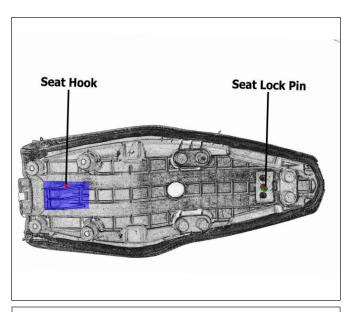
Under the seat, there is a hook and a seat lock pin, which are both important to secure the seat onto the bike.
