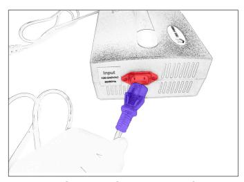
Plug the Separate Cable into the Charger
