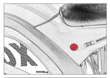
• The storage lock is located on the left side of the bike, below the seat cushion.
