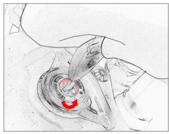
• Follow the mark on the ignition, turn the key anti-clockwise to lock the steering.
