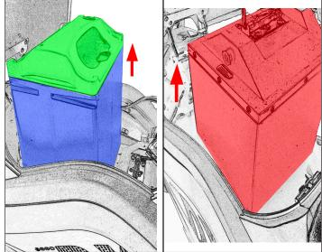
Pull out the battery box and then remove the battery. (For dual battery version, both cases will be lithium batteries.)
