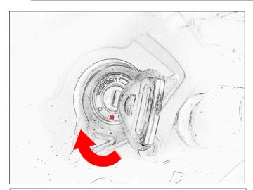
To turn on the bike, plug the key into the main ignition key hole.
