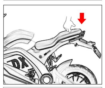
Insert the seat hook into the U shape clamp on the bike, and gently push the seat sushion down to lock it.
