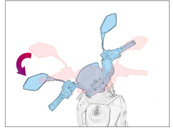
To lock the steering, turn the handlebar to the left.
