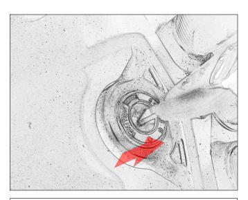
Remove the key when the steering is locked.
