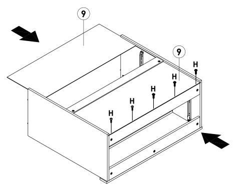
Slide down 2 pieces **Back Panel** onto **Side Panel** (**Left**) and **Side Panel** (**Right**) through the groove as shown on drawing.
