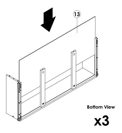
Slot Drawer Base into Drawer Side (Left) and Drawer Side (Right).
