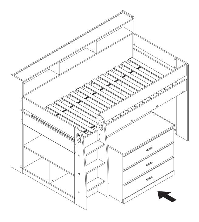
Insert **3 Drawers Chest** into undernearth the mid **Midsleeper**. Go on to complete the entire assembly.
