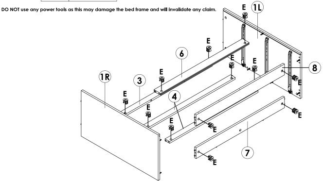
Attach and secure Front Rail (Top), Front Rail (Center), Rear Rail, Bottom Rail (Front) and Bottom Rail (Rear) onto Side Panel (Left), Side Panel (Right) and insert (E) tighten it up by using a Crosshead Screw Driver.
