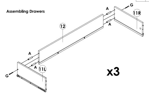
Attach and secure **Drawer Side (Left)** and **Drawer Side (Right)** onto **Drawer Rear** by using **(A)** and **(G)** tighten it up by using a Crosshead Screw Driver.
