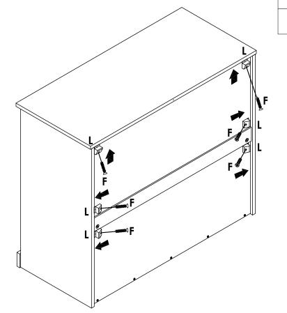
Attach and secure **(L)** on sides pointed by arrows on the drawing as shown by using **(F)**, tighten it up by using Crosshead Screw Driver.
