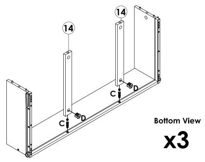
Attach and Secure **Drawer Base Support** onto **Drawer Rear**, by using **(C)** and **(D)**, tighten it up by using crosshead screw driver.
