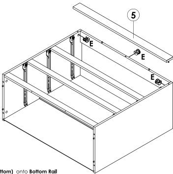
Attach and secure Front Rail (Bottom) onto Bottom Rail (Front), Side Panel (Left), Side Panel (Right) and insert (E) tighten it up by using a Crosshead Screw Driver.
