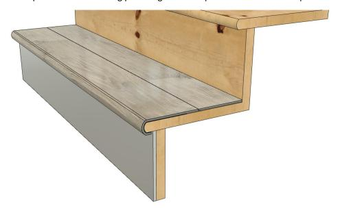
11. Adhere the riser cover to the riser to finish the step. Repeat process for remainder of steps.
