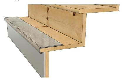
6. Mark the width of the measured stair tread to the flooring plank so that both ends of the plank will be cut off.
