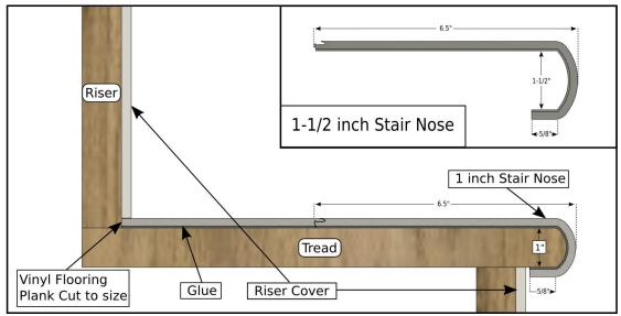
This picture depicts a side view of a stair tread and riser. The Luxury Vinyl Tread (LVT) nose piece is installed and glued into place, and joined with a piece of standard stair planking that has been cut to cover the remainder of the tread. A riser cover can then be affixed to finish the step.
