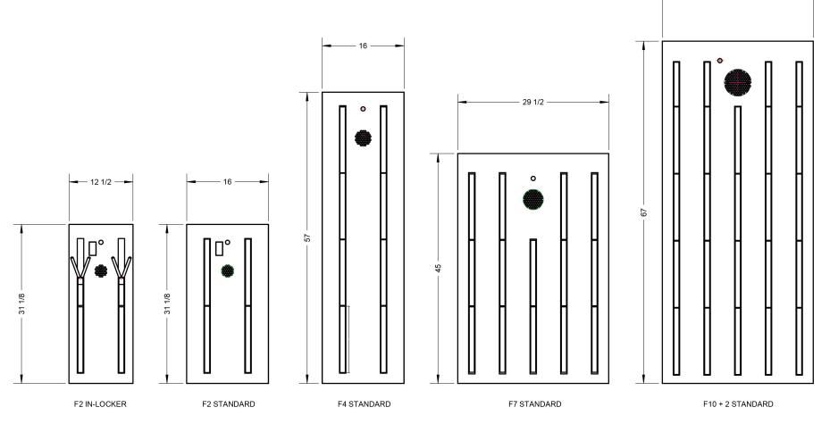
STANDARD SIZES FOR FLANGE MOUNTED IN-WALL DRYERS
