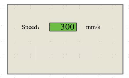
A cursor will appear when pushing  $\triangleleft$  or  $\triangleright$ . Move the cursor to the numeral area and push  $\triangle$  or  $\nabla$  to change the value. Press **ENTER** to save the change. Press **ESC** to invalidate the change and return to the main interface.
