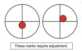
The laser mark should be near the centre of the hole. If the laser is not centred on the 1st mirror, cut the power to your laser and carefully adjust the laser tube in its brackets. This may require loosening the screws on its stand and adjusting its brace wheel. Be careful not to overloosen the screws and not to overlighten them. Only adjust one stand at a time.
