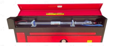
Step 4. Inside the main bay, remove the nylon cable ties from the X axis and the honeycomb table.
