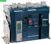
Circuit breaker frame, MasterPact NW25H1, 2500A, 65kA/440VAC 50/60Hz (Icu), 3 poles, fixed, without control unit
