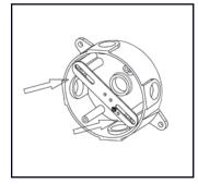
4. Install the bracket on the junction box with 2 screws.
