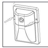
6. Attach the fixture to the bracket by using 2 sets of screws and washers, then push flat against the wall.
