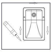
7. After the fixture is installed on the wall, fill the gap between the wall and the fixture with glue. (Only 3 mounting surfaces need to be filled)
