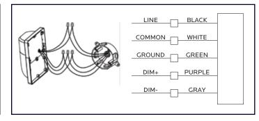
3. Make supply wire (power and dimming) to fixture wire connections as required thru splice access. Universal voltage driver allows operation at 110V thru 277V, 60 or 60Hz. 0-10V control wires must be rated for 300V minimum. For 0-10V dimming, refer to the above diagram.
