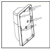
2. Fix the back cover with fixture by using the 6 screws.
