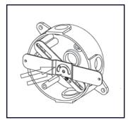
5. Use 2 screws to fix bracket after adjusting position.
