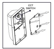
1. Loose the 6 screws on the back cover of the fixture to open the back cover and adjust the CCT switch.
