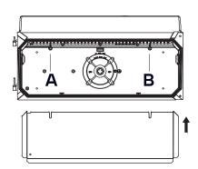
Put back the reflector and tighten the 2 screws (A/B)
