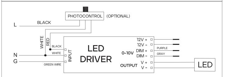
Please connect black wire from luminaire to black wire (L) of branch; connect white wire from luminaire to white wire (N) of branch; connect green wire from luminaire to green wire (G) of branch.
