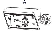
Fix the back housing to the junction box and connect wires as per the wiring diagram.
