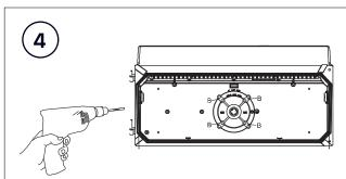
Prepare the back housing for mounting by drilling or knocking out the appropriate hole.
