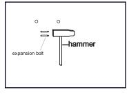
2. Drive in the bolts to the pre-drilled holes with thread outside, as shown below
