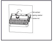
4. Fasten the screw nut clockwise with provided wrench
