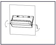
5. Rotate the light to the proper angle and fasten the screws
