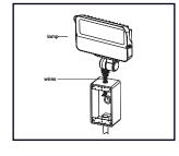
4. Use wire-nuts to connect the wires of lamp and J-box
