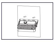
3. Make the bracket face tightly to the wall through the thread
