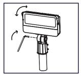
3. Adjust the lamp into desired angle
