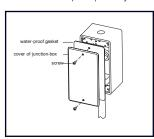
3. Screw up the knuckle mount into junction box
