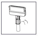
2. Tighten the screws to secure the lamp on the lamp pole
