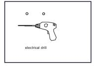
1. Mark the position of the fixing holes with fold light bracket, then drill fixingholes
