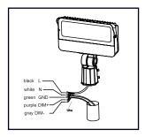
1. Loosen the 4 screws on the lamp holder, connect the wires correctly and put the wires into the lamp pole
