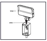
4. Use wire-nuts to connect the wires of lamp and J-box
