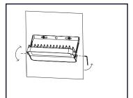
5. Rotate the light to the proper angle and fasten the screws
