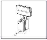
7. Adjust the lamp into suitable angle
