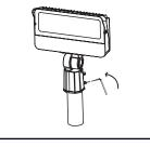
1. Loosen the 4 screws on the lamp holder, connect the wires correcity and put the wires into the lamp pole
