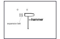
2. Drive in the bolts to the pre-drilled holes with thread outside, as shown below
