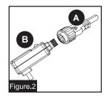
3. Connect two string lights together by pushing the male and female end connections together, ensuring the 2 pins align with the 2 holes in the receiving end, then tightening the screw-on connection cover. Ensure the last string in the series has its end cap attached. Do not connect more than 4 strings together
