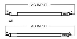
Input Voltage: 120-277V 50/60Hz
