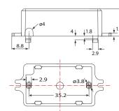
Note: Motion sensor setting and dimming setting please refer to remote control HD03R. HD02VRH Wire diameter 4mm, Standard Version Cable Length 48.5 cm(can be customized).
