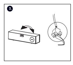
3. Open the junction box cover and remove the appropriate knockout(s). Using quick-connect push-in terminals and connect wires.
