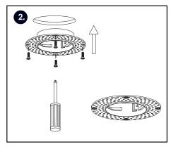
2. Fasten the trim to the ceiling with the screws.
