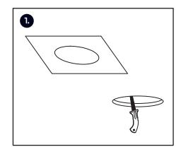
1. Determine the location for installation and cut ceiling hole in accordance with cut-hole dimensions.
