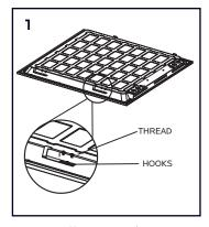
1. Turn off the electrical power, then make sure the backlit cable hooks are installed.
