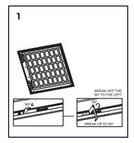
1. Remove the original ceiling tile for the backlit LED panel.
