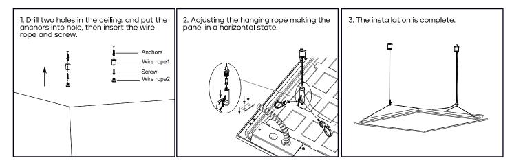
NOTE: 2X1, 1X4, 2X4: 2 PCS SUSPENSION KITS NEEDED FOR INSTALLATION
