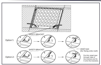
1. Use the safety brackets to secure and keep in place.
