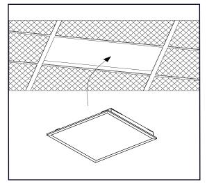
1. Replace existing light fixture from ceiling with LED panel
