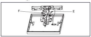
3. Connect the dimming light with P2 terminal E, and connect the power line and ground wire with the 3 hole wiring terminal F (bare copper wire to green ground wire, other wire colors match.)
