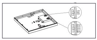
4. Turn the power switch and color temperature switch to the desired setting.
